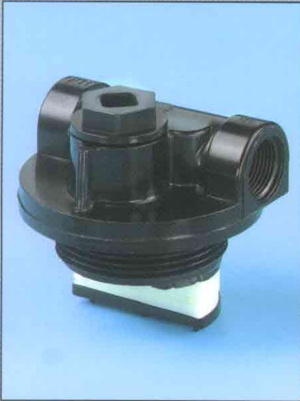
XWPE-50IS Manifold Inlet screen option 3/4" npt external 3/4" fill port w/cap Riser dia.: 1/2", 13/16" Offset Slot clearance: .012" Material: ABS
